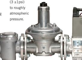
With a negative outlet pressure, the design allows the system to use a "demand" control scheme whereby engine intake airflow determines the gas flow of the engine. As engine load changes, corresponding changes in intake air volume automatically draw additional fuel into the mixer.
