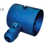
robbing throttle plate. The low restriction air-gas mixer ensures that adequate air-flow is maintained to the engine and that operating efficiencies are not compromised by installation of the device. The computer-aided-design mixer is built to aerospace tolerances using CNC machining processes and is assembled using state-of-the-art welding techniques. The finished mixer has no moving parts and once installed in the engine air-intake system
