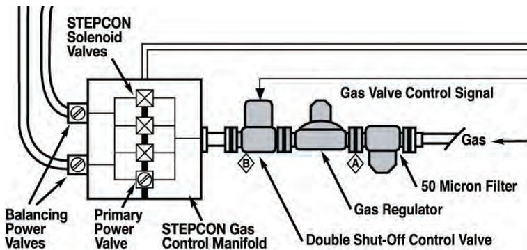
The STEPCON® enhances the bi-fuel system, allowing its application over a wider load range, adjusting the optimal substitution rate based on load with the capability to make substitution level adjustments in response to rapid load changes.
