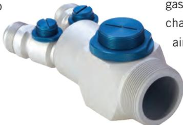
The power valve works in concert with the air-gas mixer and zero-pressure regulator to supply the required quantity of gas to the engine. Like the air-gas mixer, the gas power valve is built using computer-aided-design and CNC manufacturing and requires no routine maintenance.
